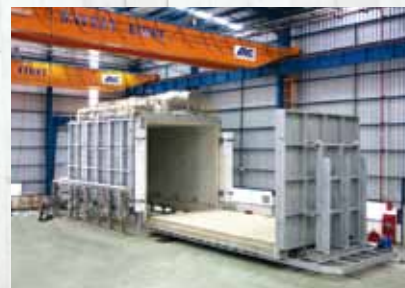
Convection type car bottom heat treatment furnace Opened
