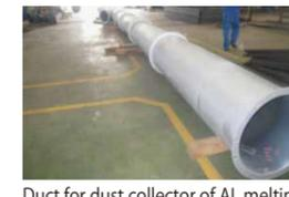
Duct for dust collector of AL melting furnace and attached structures
