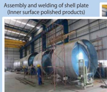
Assembly and welding of shell plate (Inner surface polished products)
