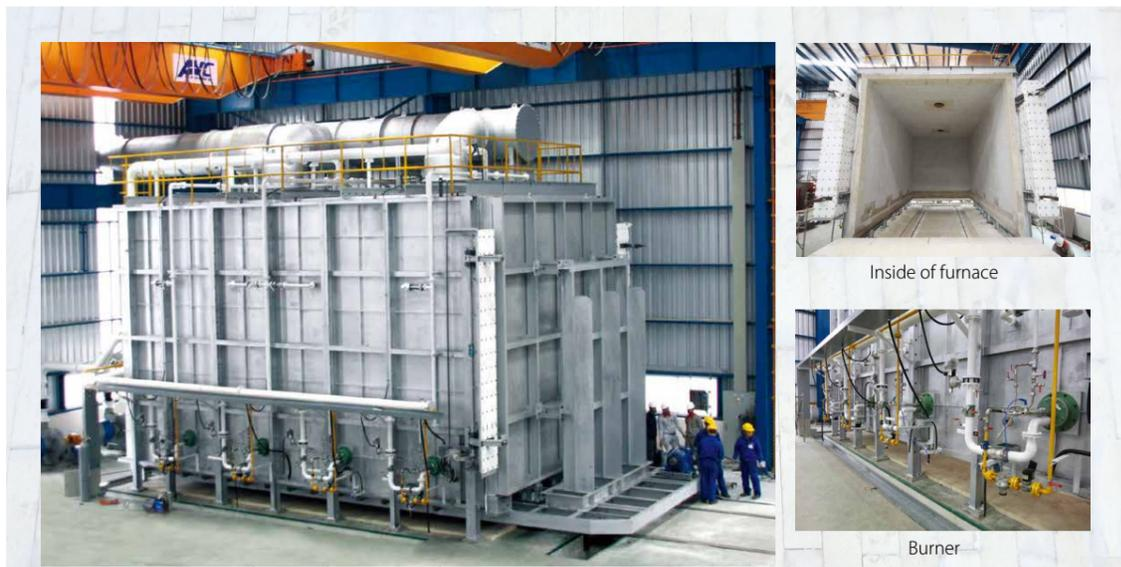
Convection type car bottom heat treatment furnace Closed
