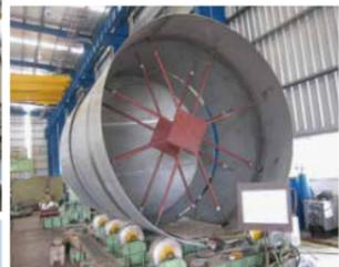
Installation of partition plate (SUS304)
