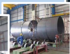
Assembly and welding of shell plate (SS400)
