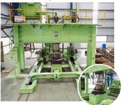
SSM (Special Spinning Machine) 3 1000ton pressing machine
