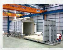
Convection type car bottom heat treatment furnace Opened
